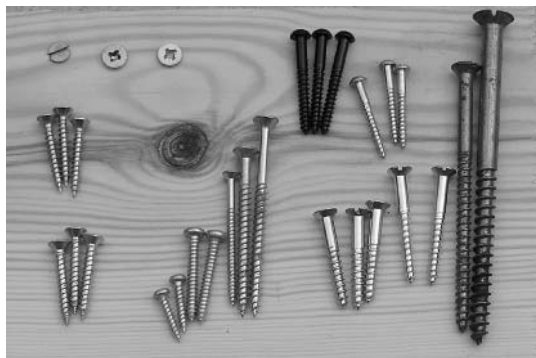
Fig. G.6 A selection of screw nails for timber
