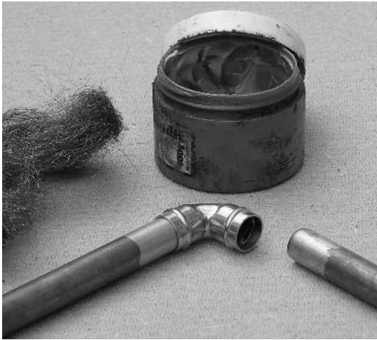
Fig. 12.3 Capillary fitting joining two lengths of pipe.
