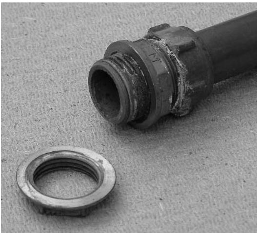
Fig. 12.8 Male iron to copper connection with a back nut.
